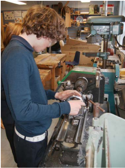
Members of the engineers using a lathe and tapping a thread.
